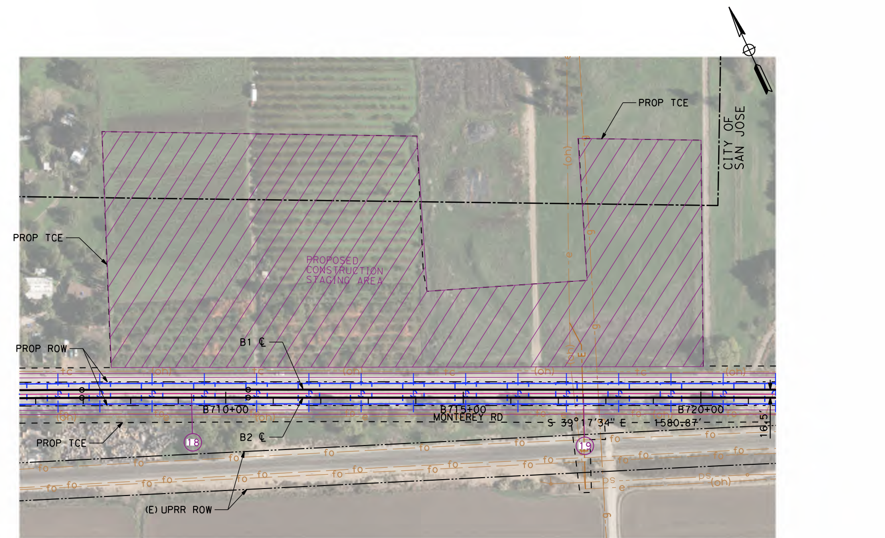
PROPOSED STAGE CONSTRUCTION STAGING AREA AT STA B707+59 TO STA B720+05 SCALE: 1"=200'
