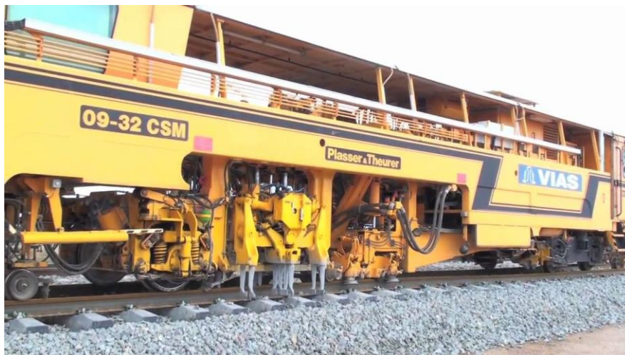
Figure 1. Tamping machine used for lateral displacements of the track between 0 and 1 ft.
