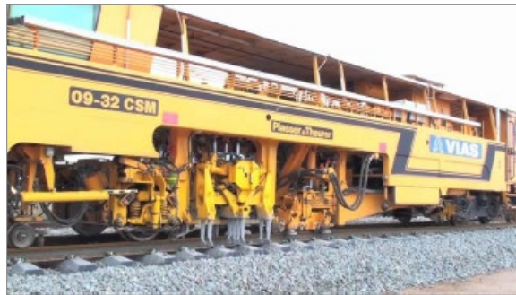
Figure 2-51 Tamping Machine for Minor Lateral Track Shifts (<1 foot)
