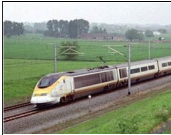
Figure 2-4 Example of an At-Grade Profile Showing Contact Wire System and Vertical Arms of the Pantograph Power Pickups
