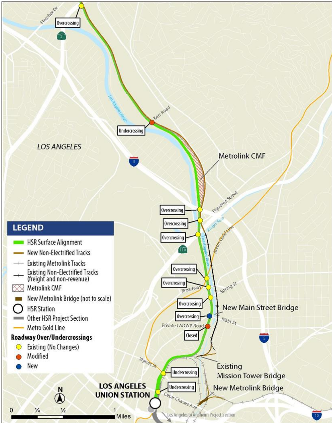
Figure 10 B-LA Alignment: SR 2 to LAUS
