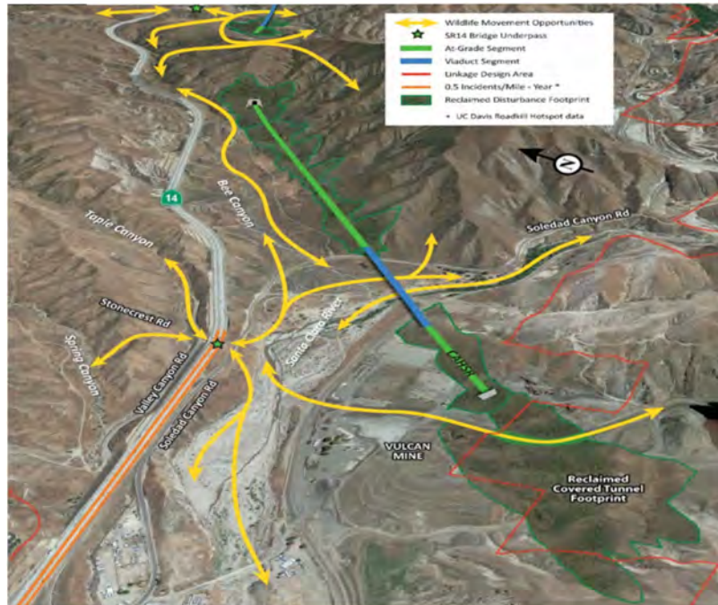
Figure 5 - Aerial photograph showing wildlife movement opportunities, looking north from Stonecrest Road, through the Linkage Design, across the SR 14 freeway corridor with UC Davis Wildlife-Vehicle Conflict Hotspots identified.
