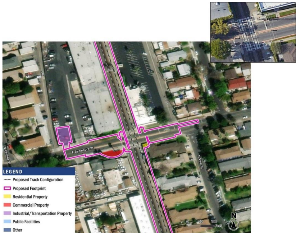
Figure 4-3 Sycamore Street Crossing Closure/Pedestrian Crossing Configuration Options
