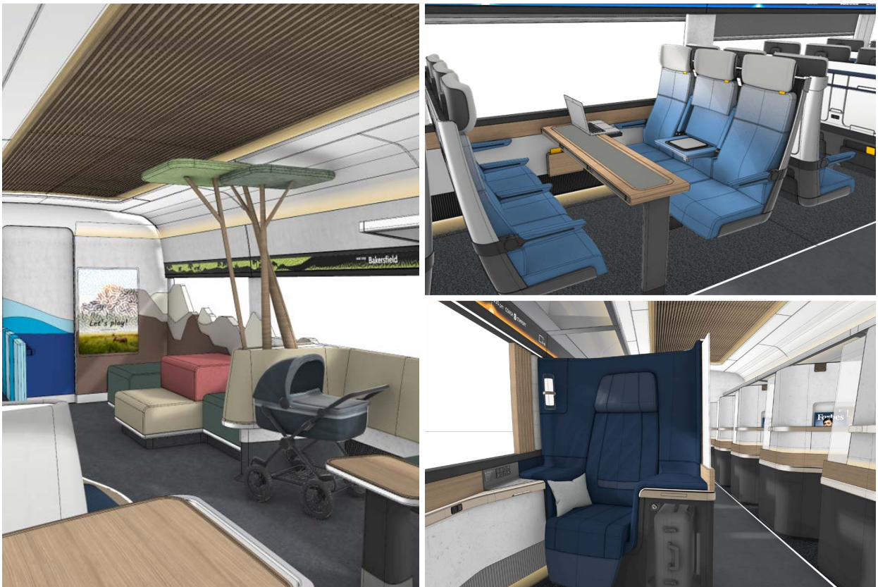
Rendering: Preliminary train interior concepts, including a family play area, general seating and premium seating
