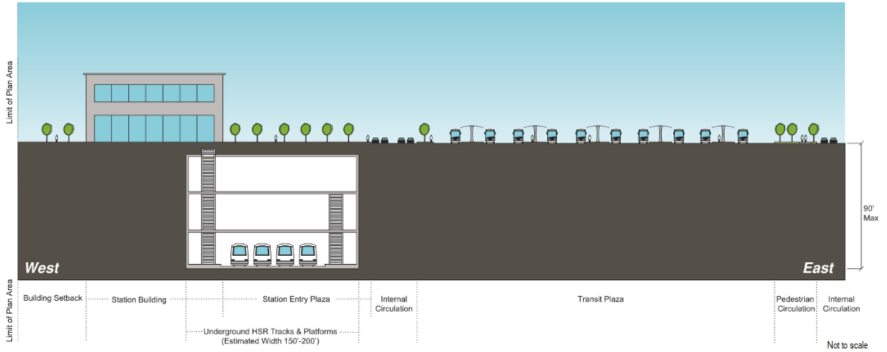
Figure 2-54 Burbank Airport Station Preliminary Station Concept Layout Plan—Cross Section
