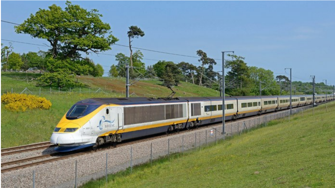
Figure 2-4 Example of At-Grade Profile Showing Contact Wire System and Vertical Arms of Pantograph Power Pickups
