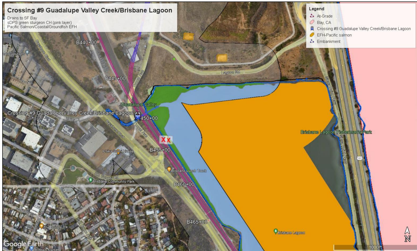
Figure 12. Guadalupe Valley Creek/Brisbane Lagoon Crossing #9. HSR to use existing at-grade tracks (maroon lines) to cross the Guadalupe Valley Creek discharge outlet into Brisbane Lagoon near Tunnel and Bayshore Boulevard in Brisbane, California, south of the proposed Brisbane LMF location. These waterways are tidally influenced and are considered sDPS green sturgeon designated critical habitat (pink layer: Bay, CA).
