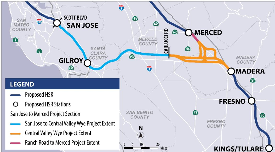
Figure 1. Geographic extent of the San Jose to Merced HSR (Scott Blvd to Carlucci Rd) Project Section route in light blue, including its westward connection to the Merced to Fresno section in the California Central Valley at Carlucci Road. The Merced to Fresno section consists of the CV Wye (orange) and its northward connection to Merced (maroon) (Authority 2020c).
