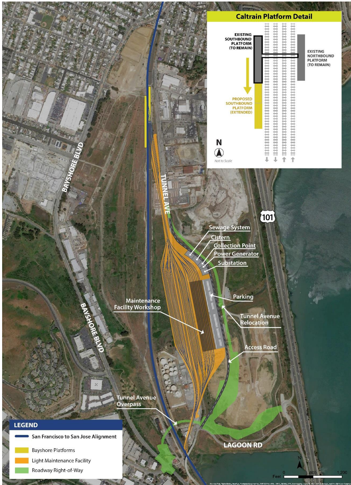
Figure 2-12 East Brisbane Light Maintenance Facility Layout—Alternative A
