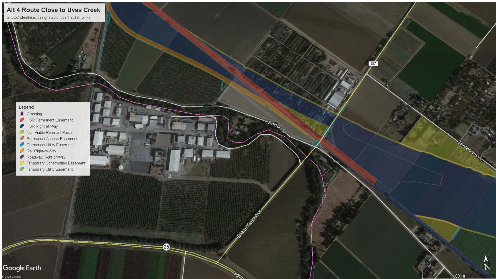
Figure 19. Close-up of HSR elevated viaduct/berm route and maintenance facility ROW (dark blue) with temporary construction easement estimates (yellow) relative to S-CCC steelhead designated critical habitat (pink line) in Uvas Creek. Electrical interconnections in teal.
