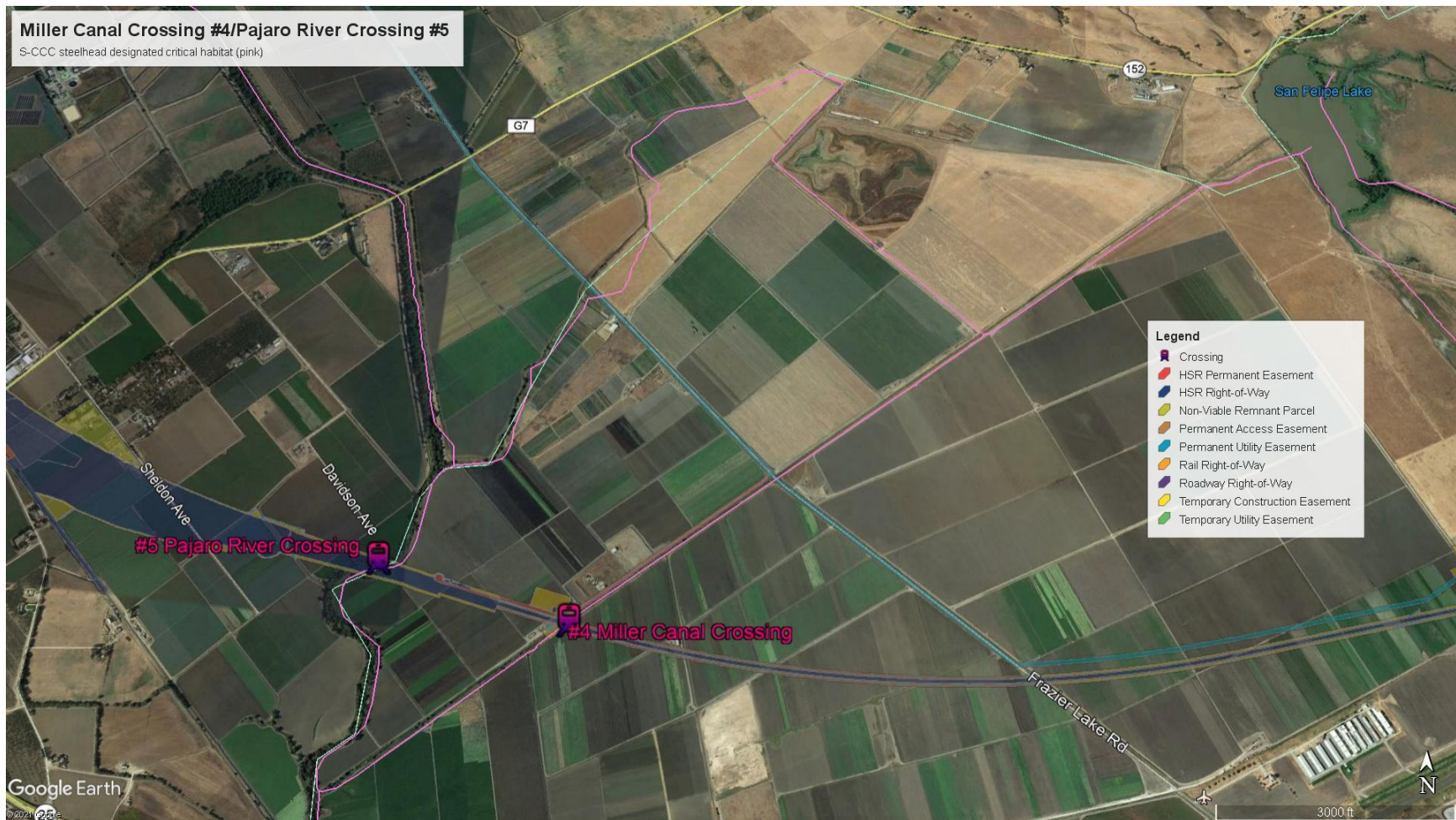
Figure 16. Miller Canal crossing #4 and Pajaro River crossing #5 by HSR elevated viaduct and maintenance facility ROW (dark blue) with temporary construction easement estimates (yellow) relative to S-CCC steelhead designated critical habitat (pink line). Electrical interconnections in teal.
