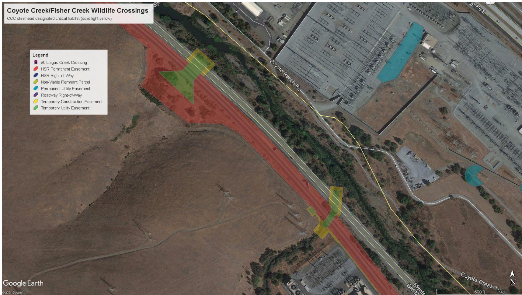
Figure 22. Close-up of Coyote Creek and HSR elevated viaduct and ROW (red) and planned wildlife under-crossings (green) with temporary construction easement estimates (yellow) relative to CCC steelhead designated critical habitat (light yellow line) near Monterey Highway/Old Monterey Highway/Highway 101.
