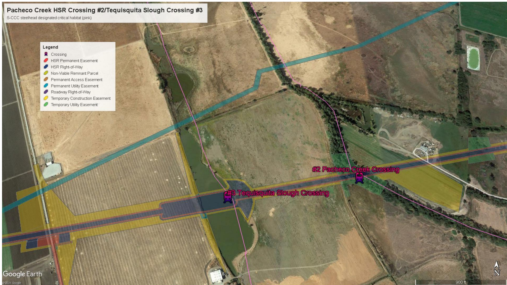
Figure 15. Close up of Pacheco Creek Crossing #2 and Tequisquita Slough Crossing #3 by HSR elevated viaduct/berm and ROW (dark blue) with temporary construction easement estimates (yellow) relative to S-CCC steelhead designated critical habitat in the Santa Clara valley floor (pink line). Electrical interconnections in teal.
