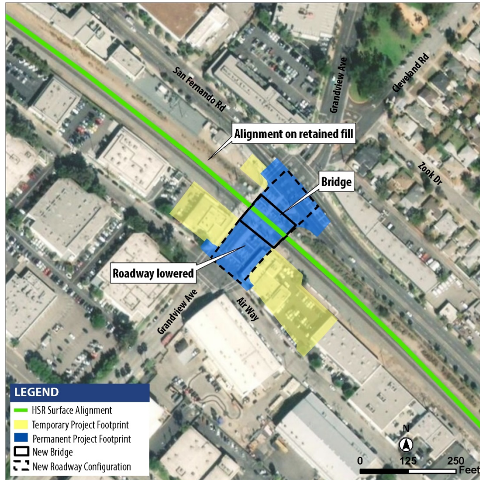
Figure 2-17 Grandview Avenue Grade Separation Footprint
