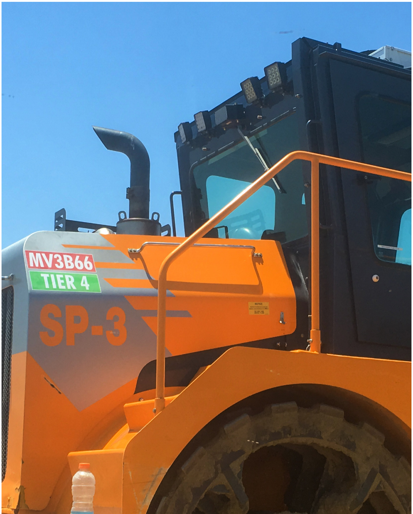
PHOTO: Tier 4 emission standards require substantial reductions of nitrogen oxide (NOx) and particulate matter (PM), and place more stringent limits on hydrocarbons (HC).
